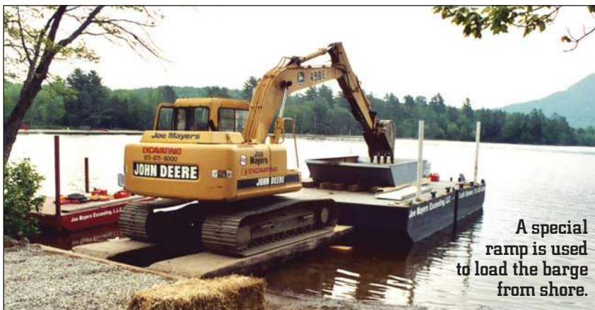
**A special ramp is used to load the barge from shore.**
