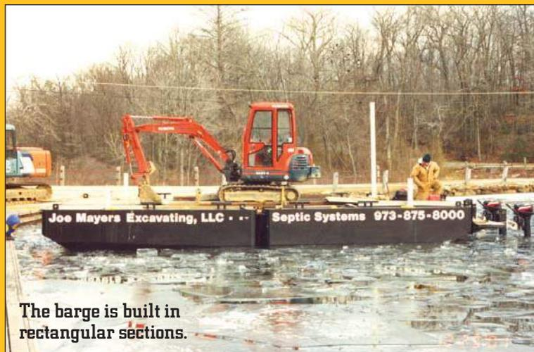
The barge is built in rectangular sections.
