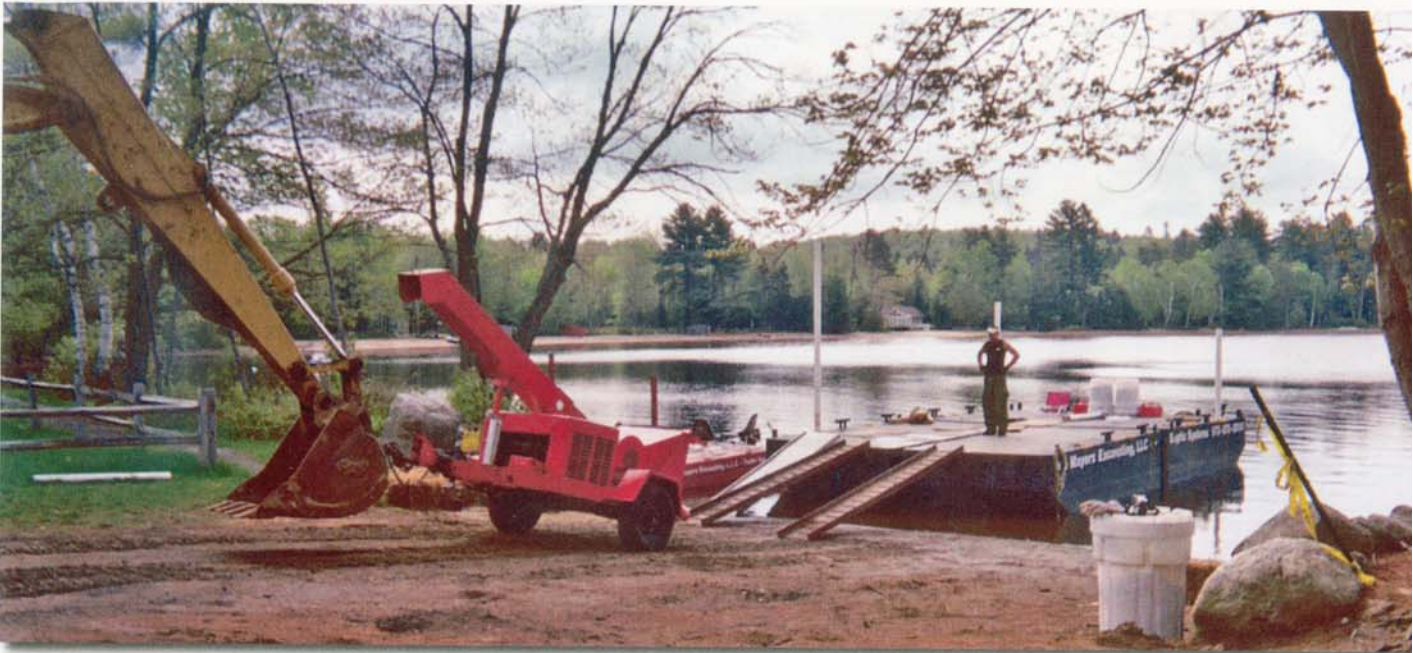
Getting ready to load wood chipper onto barge with excavator for much needed work on the island. The wood chipper is towed off barge and around the island with rubber tracked dump trucks.
